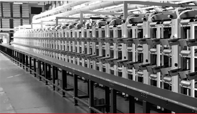
WinTape showing parking positions and transport belt
